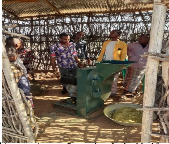
Preparation of animal feed from Prosopis feed using Hammer mill.
